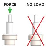
2. <u>No Side Loading:</u> Applied force must be directed upon the actuator's piston. Skewed loading may bend the piston, inhibiting its ability to retract back into the guide.
