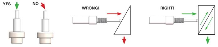
3. <u>Deadheading:</u> Not accounting for the total stroke length of the actuator's piston throughout this application range. If the full temperature range stroke is inhibited, the piston movement stops, and the internal cup pressure starts to increase. With enough restrictions on piston extension, the actuator's internals can be permanently damaged.
